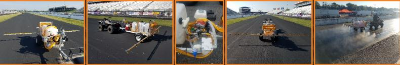
Sprays 2.5' 5.5' 8' Or 14' wide, ability to adust width on the fly. One man operation
